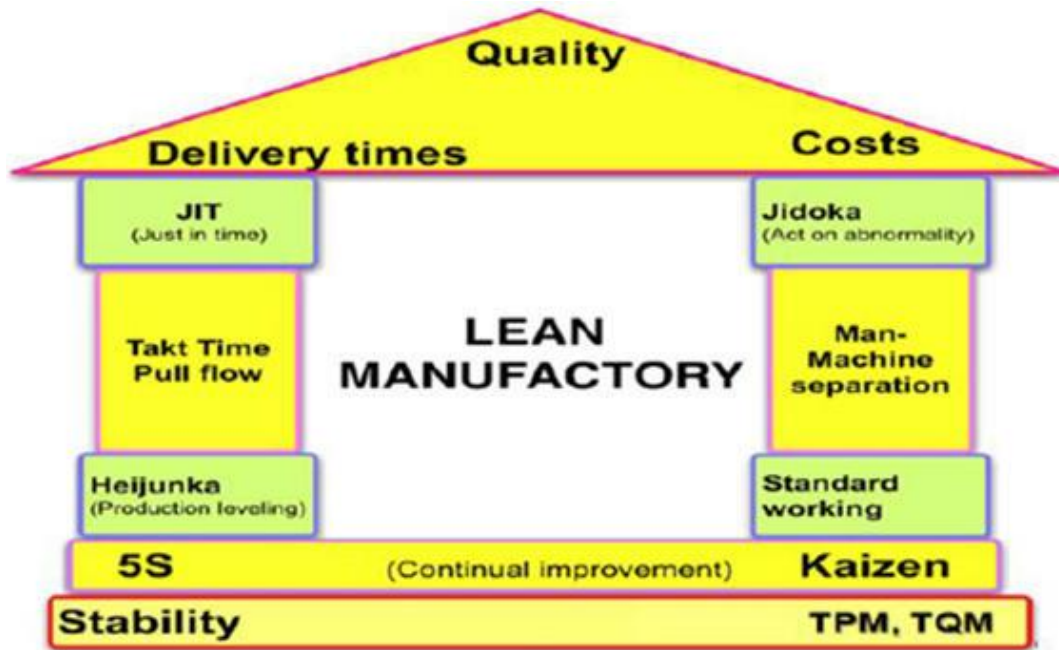
Figura 2 Estructura del Lean Manufacturing
